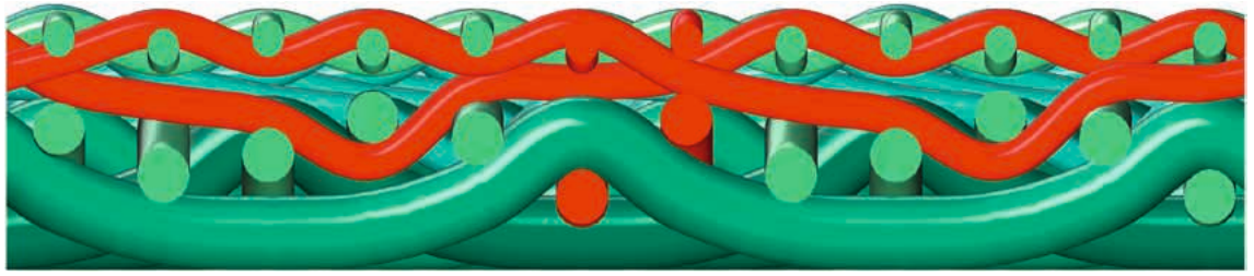
Fig 1: Standard SSB with paired binder yarns and higher void volume.
