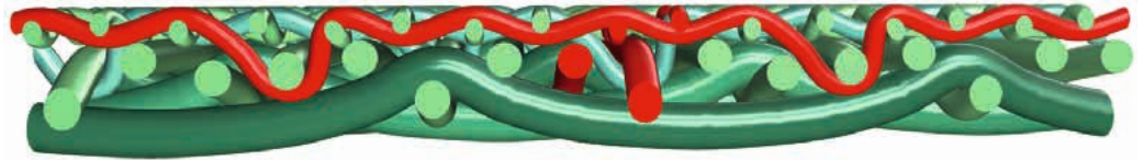
Fig 2: Primoselect concept with only a single binder yarn: Lower void volume, reduced caliper, faster dewatering.
