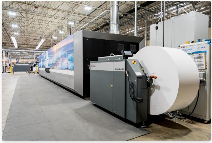
TECNAU REVOLUTION 50 ROLL-TO-ROLL, UNWINDER U50 AND REWINDER R50, IN LINE WITH CANON PROSTREAM 1800.
