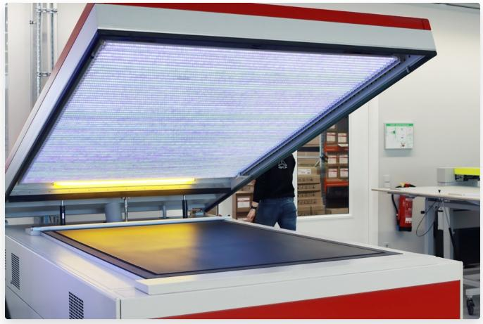
UV EXPOSURE UNIT WITH SHINE LED LAMPS.
