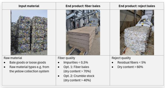
☑ INPUT AND SEMI-FINISHED MATERIALS AS SEPARATE OUTPUT FRACTIONS: CELLULOSE FIBERS AND ALMOST FIBER-FREE PLASTIC FOILS.
