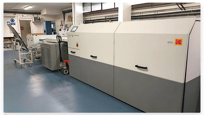
☐ GRAFICHE MILANI PURCHASED A KODAK MAGNUS Q800 PLATESETTER WITH X-SPEED AND AN AUTOMATIC DUAL MULTI-PALLET LOADER (MPL) THAT CAN HOLD TWO PALLETS WITH EACH UP TO 1,500 PLATES.
