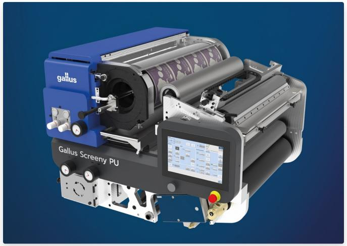
☑ THE SCREENY PRINT UNIT SCREEN PRINTING UNIT IS AVAILABLE IN PRINTING WIDTHS OF 340MM (13"), 440MM (17") AND 580MM (23").
