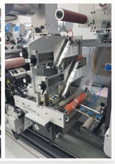
SCHEMATIC WEB PATH: THE SEPARATED NARROWER WEBS ARE ROUTED ON TOP OF EACH OTHER TO FORM THE MULTILAYER LABEL USING
