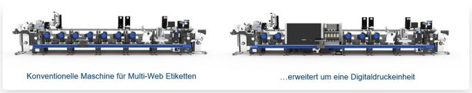
THE "SYSTEM TO COMPOSE" ENABLES THE LABELMASTER SERIES TO BE RETROFITTED FOR MULTI-WEB LABELS.
